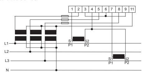
The following diagram shows a 3-element transformer connected meter with 2 current transformers and a floating neutral:
