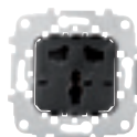
British standard socket outlet - 2M Rated voltage: 250 Vac. Rated current: 13A. Type G: 2P + E. Without switch. Shuttered for child safety. Screw terminals. Cover plate for British socket type: 8537.
