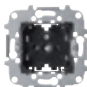
French/Earth-pin socket outlet for plain covers Rated voltage: 250 Vac. Rated current: 16 A. Type E: 2P + E. Shuttered for child safety. Screwless terminals. Included: fixing claws. Cover plate code: 8587.9.
