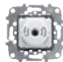
Rotatory room thermostat with floor sensor Rated voltage: 230 Vac ; ±10 % - 50/60 Hz. Load power: 2.300 W. Load type: floor heating resistor. Control temperature: +5 °C to +45 °C (Set point). OFF state: At OFF position, the thermostat is off, so that it does not address the temperature measured by the floor temperature probe. The relay output contact is open. Temperature accuracy: 0,5 °C. Hysteresis: 0,5 °C. Floor temperature sensor: NTC, 10KΩ at 25°C, -40°C to 80°C. Double isolated cable, 4m length. LED light indication: Red and green. Ambient temperature: -20 °C to 45 °C. Without fixing claws. Cover plate code: 8540.9.
