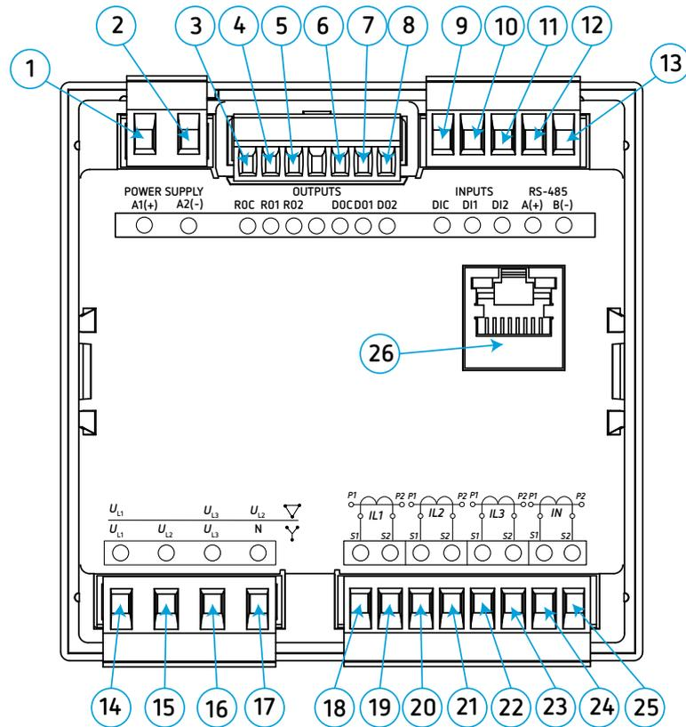
Figura 2: Bornes del CVM-C11-ITF-IN-ETH-ICT2.
