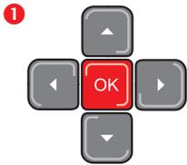
Switch on the configuration tool by pressing the OK button for 2 seconds.
